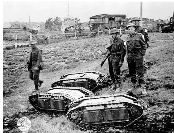
British soldiers with captured German Goliath remote-controlled demolition vehicles (Battle of Normandy, 1944)
